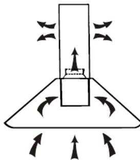
Activated carbon filter can be used to trap odors.
